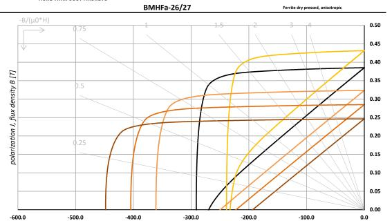
demagnetization field H [kA/m]
