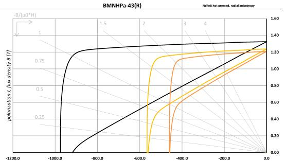
demagnetization field H [kA/m]
