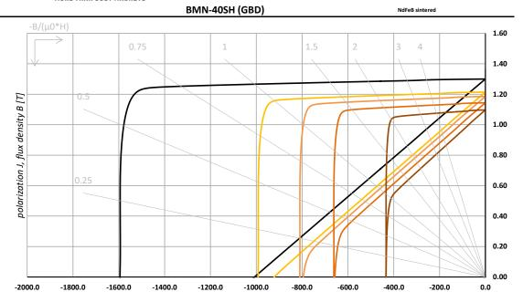
demagnetization field H [kA/m]
