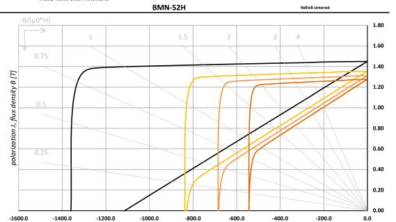
demagnetization field H [kA/m]
