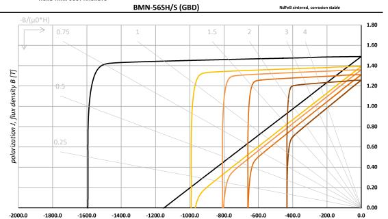
demagnetization field H [kA/m]
