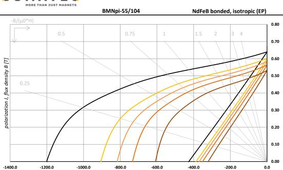
demagnetization field H [kA/m]
